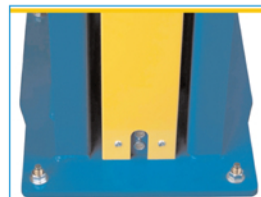
Pallet sensor to detect pallet presence before extending forks
