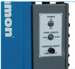
Operator console mounted to back of mast
