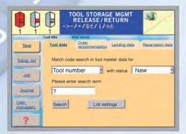
Main menu of the MP 12 N-S with integrated tool management module
