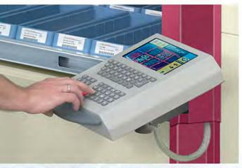
The Hänel MP 12 N-S top controller with container photo view
