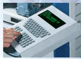
MP 12 D-S device controller with VF display with 4 x 20 characters for high-contrast display
