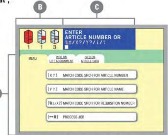
Quick-start user interface for storing and retrieving parts by article number. Function keys for the different match code searches and for processing jobs by keyboard or via the touchscreen
