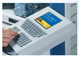
MP 12 D-S device controller with CSTN colour display and 320 x 240 pixels
