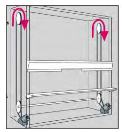
Dual motor design provides more power with redundancy for longer life and emergency operation.
