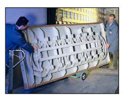
Pre-assembled Rotomat sections make assembly faster and maintain a higher level of strength and quality than multiple components assembled on site.
