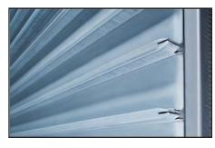
Slot walls eliminate fixed location assignments and the need to manually make profile changes.
