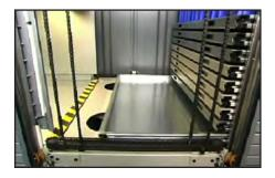
Four rollers on the outer edge of the transporter provide 4 points of support to avoid tilting and problems from imbalanced loads.
