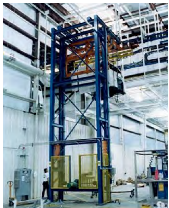
Power & Free "Lowerator" for truck cab system from paint to assembly.
