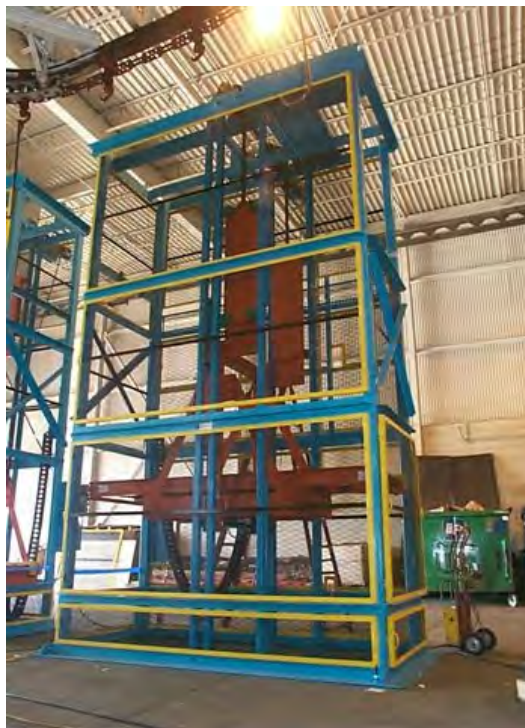
Reciprocating lift set up in our shop for testing. Intermediate sections will be installed at job site for final height of lift.
