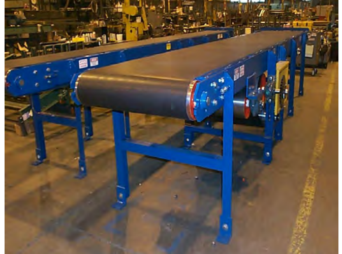
Typical PVC belt conveyors. This feature center drives so fixed ends are possible.
