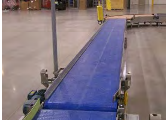
Plastic belting used for delivery and assembly. Though more costly than standard belting, this new belting offers many unique advantages.
