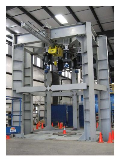
HECO Pacific Mfg. Inc. has built various test stands up to 1,000,000 lbs, used to test structures and specialty items. Systems are built to very tight tolerances with numerous critical welds and special fabrication techniques. This unit included an object monorail hoist that was fit in between the very large computer controlled jacks.
