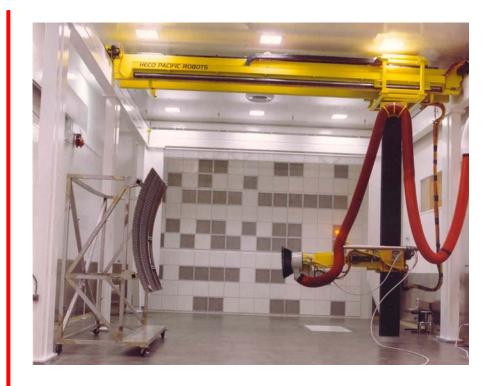
The special cleaning robot was designed and built by HECO Pacific. It is used to clean high dollar satellite fairings with CO2 pellets. The system was controlled and automated using special software and computers. The system included the self supporting runway and all precautions for a Class 10,000 clean room. Here are some the special features of our system:
