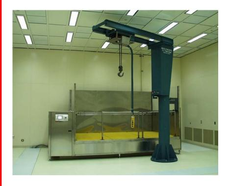
HECO Pacific Mfg. Inc. has supplied a number of special double boom low headroom jib cranes for customers around the country. These cranes can be used in specialized facilities with clean room requirements. Here are some of the special features we offer.
