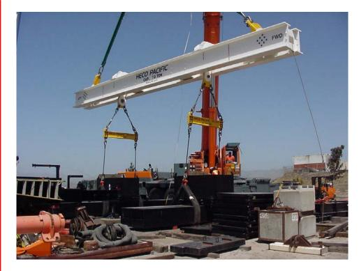
HECO Pacific Mfg. Inc. has built specialized spreader bars and below the hook devices for many application. The unit above was a 250 Ton spreader bar designed for the adjustable handling of solid rocket motors. We can provide a wide range of specialized products for any industry. Here are the types of features we offer.
