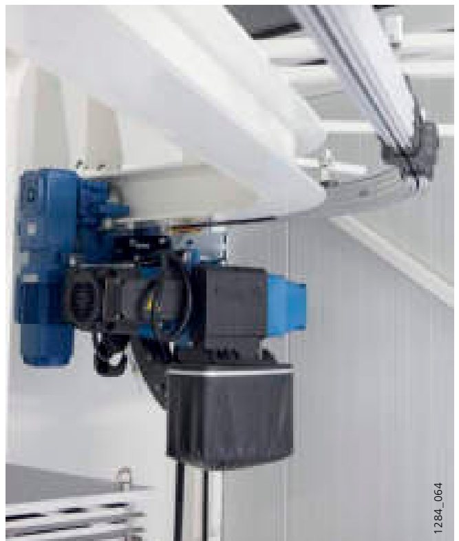
EKDDC articulated monorail hoist (low-headroom design)
