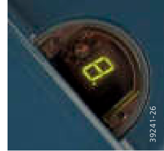
39241-26 Display for elapsed operating time counter and operating statuses
