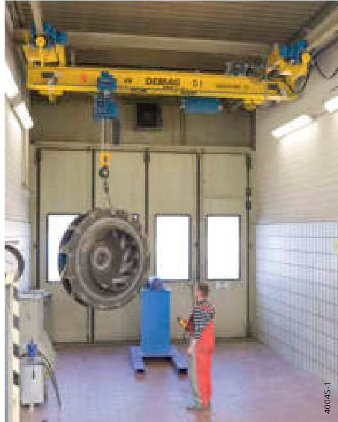
Minimum travelling chain hoist approach dimensions thanks to suspension crane end carriage based on DC chain hoist trolleys
