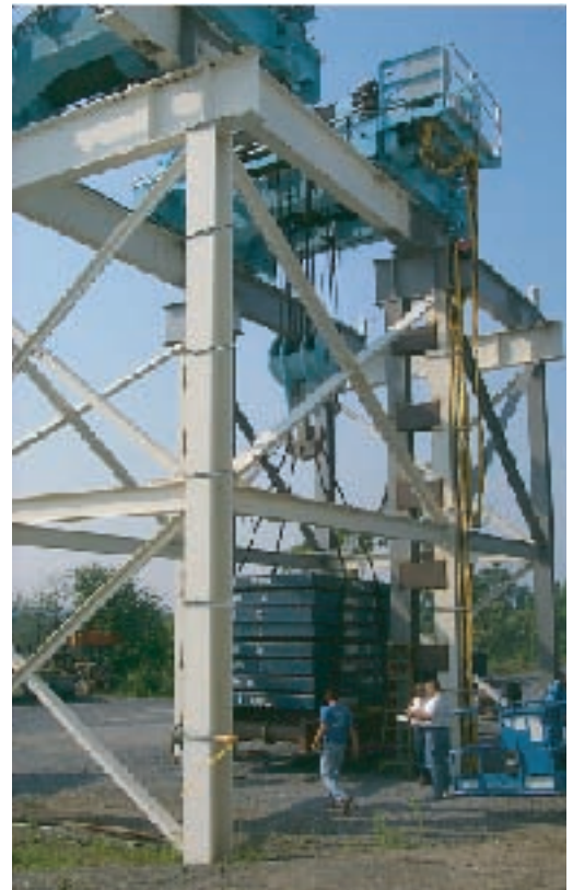
Load Testing a Trolley in our Test Tower
