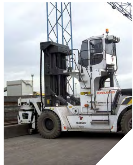
Middle: Coil stacker (40 T). Below: Bloom grab truck (20 T).
