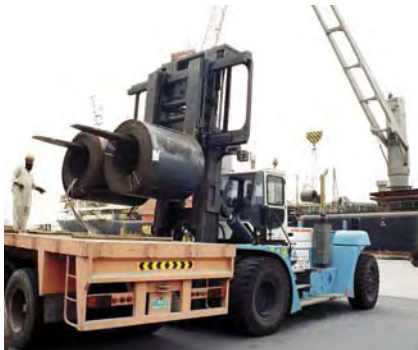
Middle: Steel magnet truck (52 T). Below: Double coil truck (32 T).
