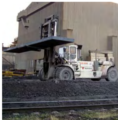
Middle: Plate stacker (45 T). Below: Slab truck (52 T).
