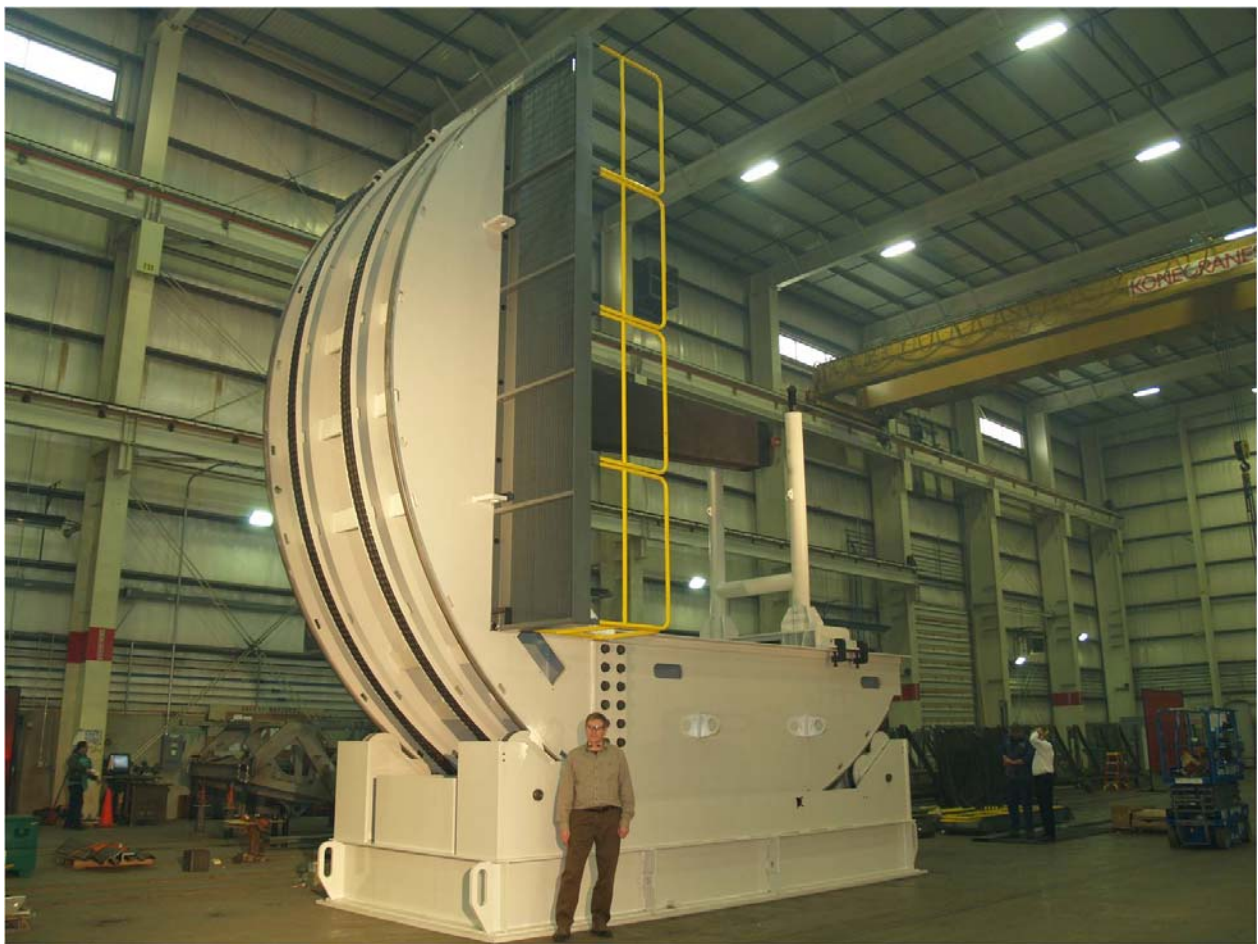
The upender is over 28 ft tall when fully upright.
