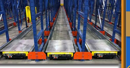
Frazier's optional No Bottom Beam design allows for floor levels to be cleaned more easily.
