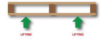
Four heavy duty ball bearings on each corner of the platform working with a screw-drive lift system respond to raise the deck lid up. The deck lid as a whole picks up the load, so that center stringers or blocks on pallets directly transfer the lifting force to the entire pallet. Lift performance is not dependent on bottom board strength.
