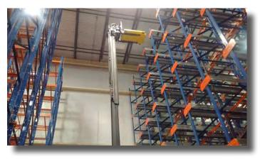
Each Pallet Mole® unit contains magnetic latches on its bottom. These allow an operator to safely lift and move the unit at any height from one position of the system to the next without fear of dislodgement.
