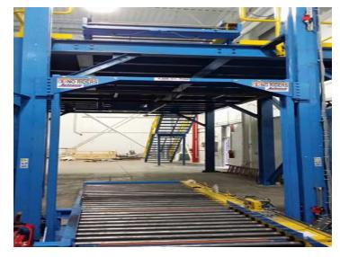
operation where the contents are then dumped into a hopper below the mezzanine level. The contents are then pneumatically blown into an adjacent injection molding room. The empty totes are then returned to the main floor by a second lift and the process is repeated.
