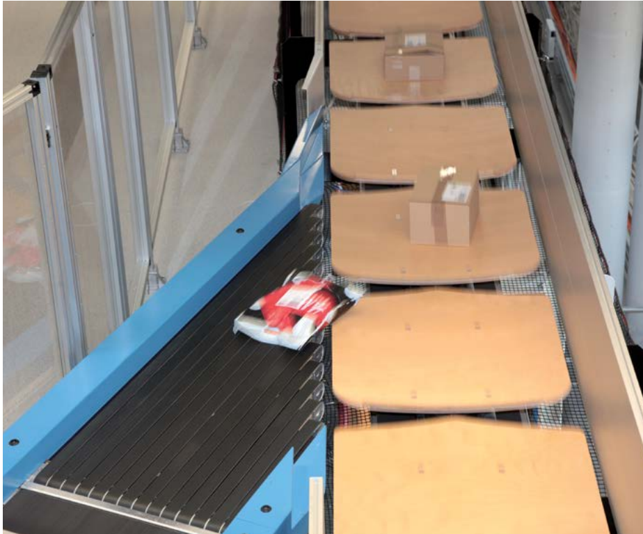
The BEUMER BS-7 Tilt-Tray Sorter is a low cost but durable mechanical tilt-tray sorter perfect for high volume shipping sortation of large retail boxes and small flat poly bags for e-commerce all on the same system.
