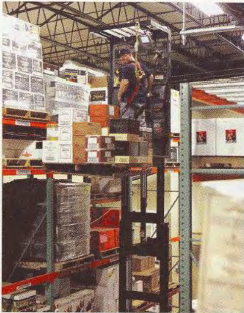
An order selector on a man-up lift truck picks cases from pallets.
