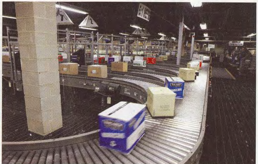
After the combiner (below), cartons are sorted to one of more than a dozen shipping doors.
