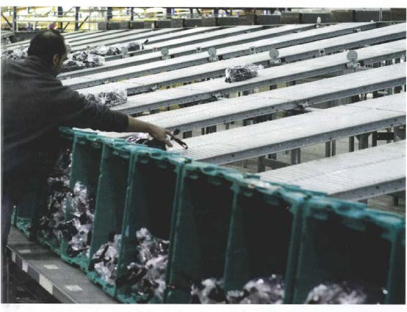
remove the garments from the boxes and separate them by type—pants, coats, shirts, vests, and so on. The workers then place the loose garments onto a belt conveyor supplied by FKI (now Intelligrated). The conveyor transports the garments to a receiving station, where an operator removes each item and scans the permanent bar code sewn onto the garment. This logs the garment back in as a receipt.
