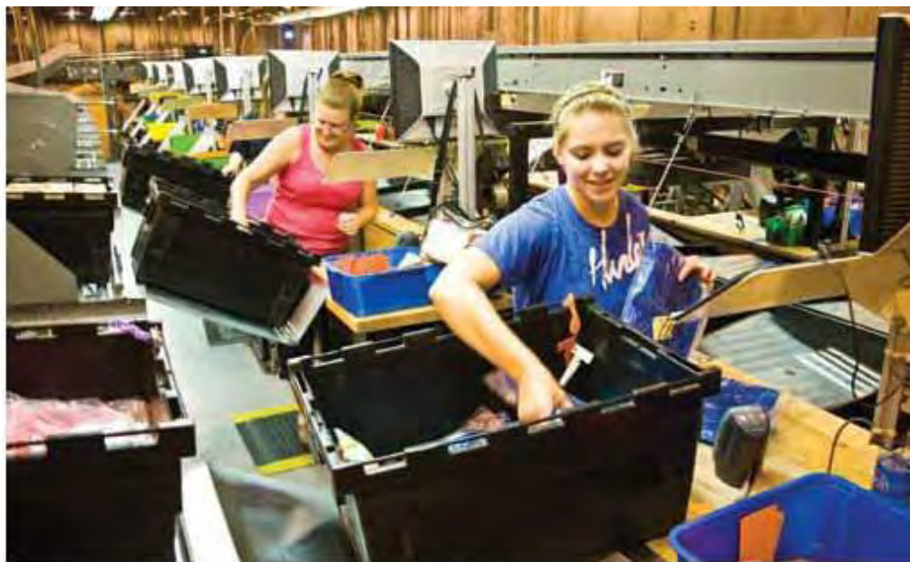
Items are picked to totes from a number of different picking zones and then conveyed to one of the sorter induction areas, where they are placed on the tilt tray sortation system.
