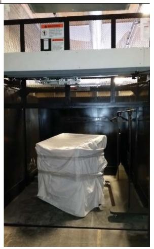
Global Industrial, a material handling products provider in the Milwaukee area, suggested that Hooge consult with PFlow Industries, a leading manufacturing of vertical lifts, also known as Vertical Reciprocating Conveyors (VRCs).
