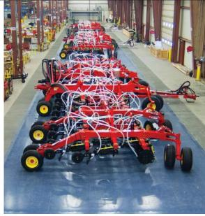
would be pushed along on rails by hydraulic cylinders. As the carts reached the end of the line, the completed tillage equipment would be rolled off from the assembly system. The carts would then be lowered, and transported underneath the assembly system back to the front of the line to be reused.
