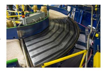
Combined with DuraSurf STS, the e-saver belt reduces the level of friction to a point where running the conveyor—even during peak energy usage—will result in savings on electricity with a favorable return on investment. Additional savings are possible because of the belt's increased durability, which results in fewer belt replacements. Finally, the e-saver belt is environmentally friendly, reducing CO<sub>2</sub> emissions.
