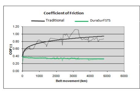
Tests conducted revealed a 68% decrease in the coefficient of friction when using Habasit's DuraSurf STS product versus a standard conveyor without DuraSurf STS.
