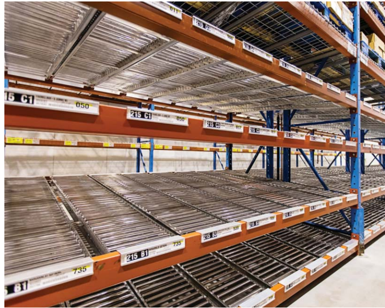
UNEX developed this unique label holder for Flow Bed lanes because stock can change so quickly at Pine State Trading Co. The labels allow order pickers to clearly see which items are stored in various lanes, and the labels can be switched out easily as SKUs change.
