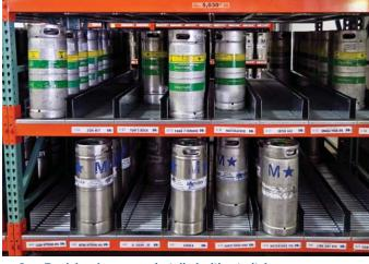
SpanTrack keg lanes were installed without pitch. The rollers assist the operators with picking/loading from either side of the rack.
