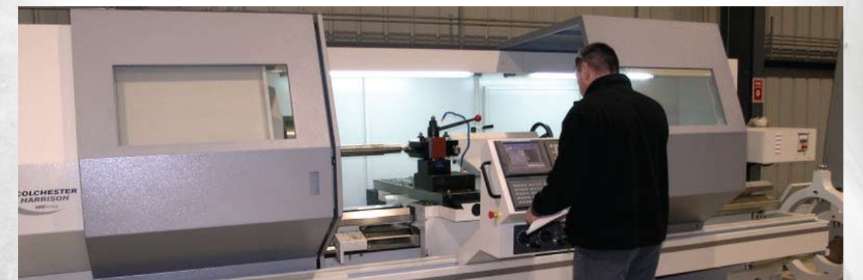
CLAUSING/HARRISON ALPHA 1800SLB X 96" CNC/ELECTRONIC LATHE: This horizontal lathe is fully automated. Once parts are programmed and stored in memory, there is no setup other than placing the part in the spindle.
