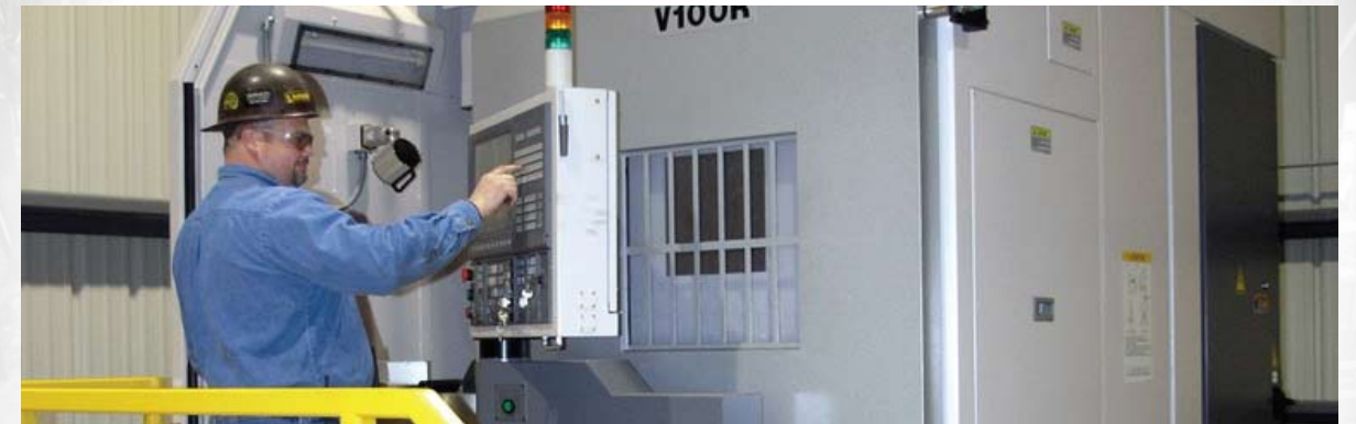
OKUMA V100R VERTICAL SPINDLE 2-AXIS CNC TURNING CENTER: This machine produces wheels, sheaves and other cylindrical parts quickly and accurately.
