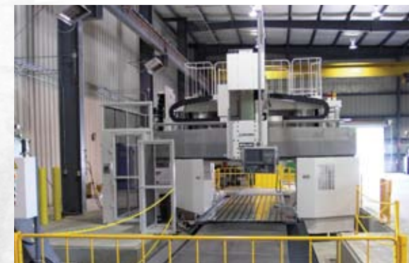
OKUMA MCR-A5C 5-AXIS DOUBLE COLUMN CNC MACHINING CENTER: This state-of-the-art piece of equipment can completely machine five sides of a part without repositioning. Once programmed, it changes between vertical and horizontal heads as needed. The heads then select the proper tool from the tool storage magazine and go to work, all without operator intervention.
