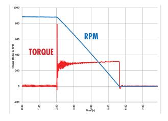
DC Magnet Brake Torque Curve
