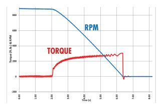
AC Thruster Brake Torque Curve
