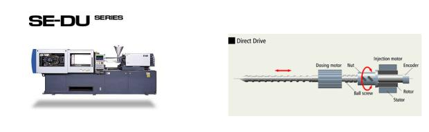
Fig.9 Injection Machine Sumitomo SE-DU Series
