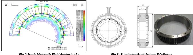
Fig.2 Static Magnetic Field Analysis of a Sumitomo DD Motor (3.3kW, 500r/min.)
