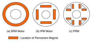
Fig.1 Rotor Construction of Permanent Magnet Motor
