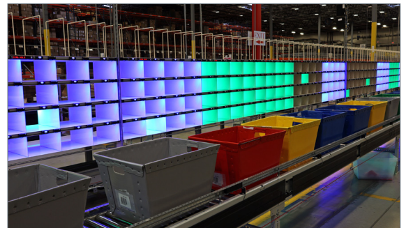
Two-sided put wall for sorting and packing.
