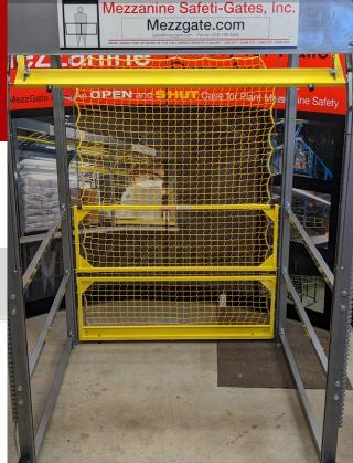
When the pallet drop area is being loaded, the ledge gate is open and the netting compacts into the system, clearing the way for pallets to be moved into place. After loading is finished and the pallet area is ready for picking, the ledge gate closes and the netting extends from the deck to the top frame of the gate, providing full length coverage to prevent products from falling, decreasing the risk of damage while being picked or moved from the area.
