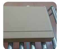
4. Upper flaps sealed with glue.
