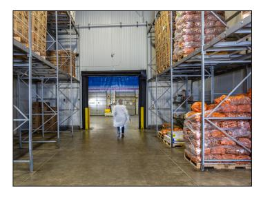
For example, the large door openings that service the threshold from the processing area to the cold loading dock area support one-way traffic. One door is meant only for forklifts to enter the dock area, while the other door is for exiting the dock area. However, if one of the doors were to become inoperable, the openings are larger enough to support two-way traffic.
