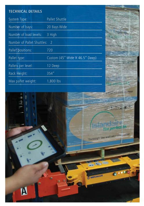
dimensions of the pallet that Islandaire is using and the model of Pallet
