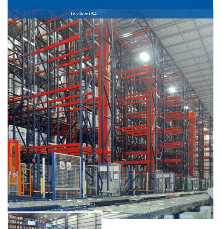
Interlake Mecalux has built a new Automated Storage & Retrieval System (AS/RS) for Next Generation Films with a storage capacity for more than 15,400 pallets of different sizes and turnovers. The installation is managed by the efficient Easy WMS warehouse management system by Mecalux, capable of maximizing the productivity of all operations being performed.
