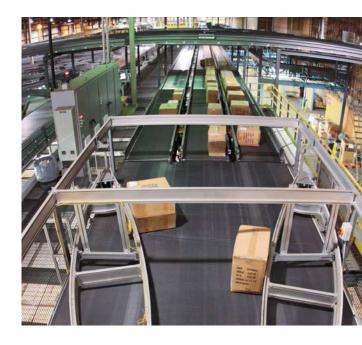
conveyor, powered roller conveyor, chain transfers, belt curves, chain driven live roller and air assisted sortation.
