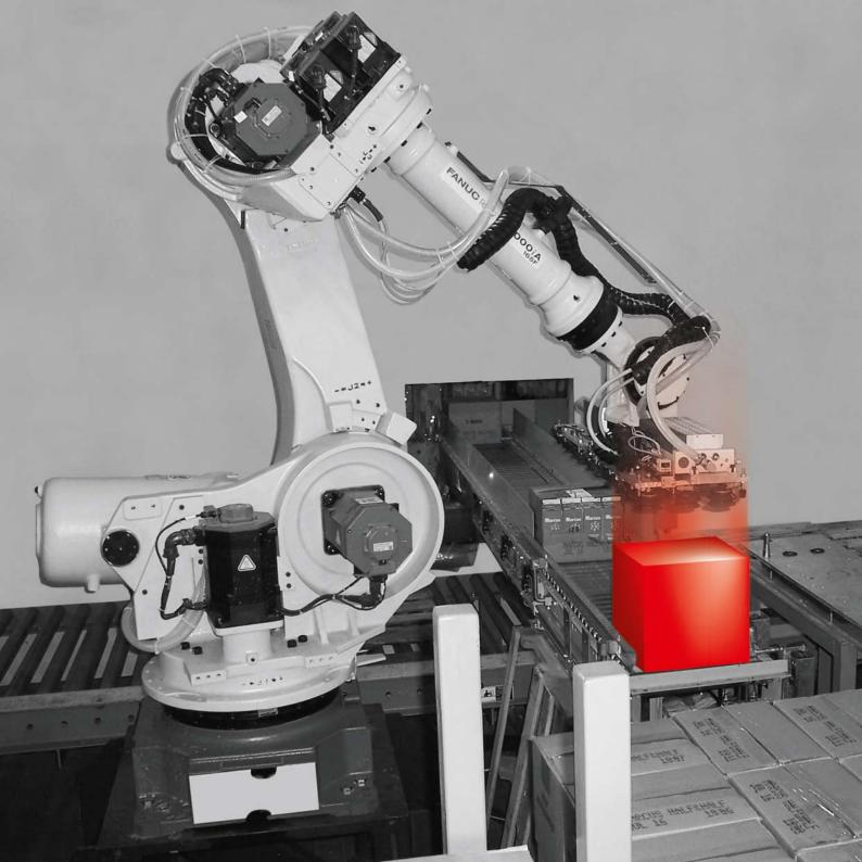
viastore specializes in total integration, handling each project from start to finish including robotic simulation, calibration, programming and maintenance. The key to any robotic application is the end of arm tooling (EOAT). Tooling can be designed to handle a wide variety of products or loads. viastore excels in designing and building the end of arm tooling to fit specific applications.
