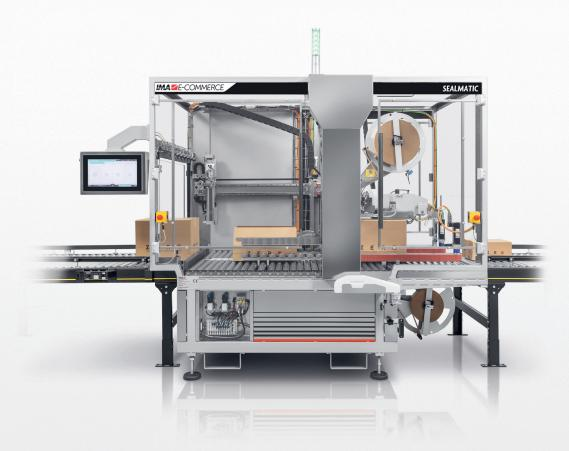
E-CO Flex SealMatic is a fully automated case sealer to process FEFCO 201 boxes, automatically adjusting its mechanical movements according to the case size. It is equipped with sustainable water-activated tape technology to seal cases on top and bottom at high speed, up to 20 boxes per minute, without the need for operator intervention.
