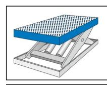
Tabletop made of 2,5 mm aluminum plate
