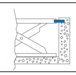
Tabletop secures in place via 4 bolts, with pit frame, operates via manual push button control, position of bolts in the long sides.
