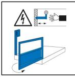
Outward-opening door in the railing, with electric and mechanic locking system. Doors open only allowed points.
