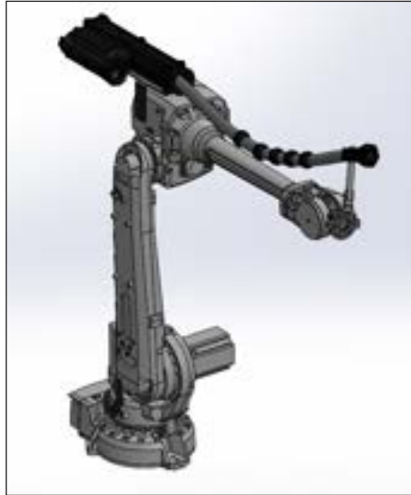
24.48.321.01 Complete robotic dresspack, Axis 3-6, TecBox retraction system, 400mm stroke, high-flex conduit with ID 36.7mm
