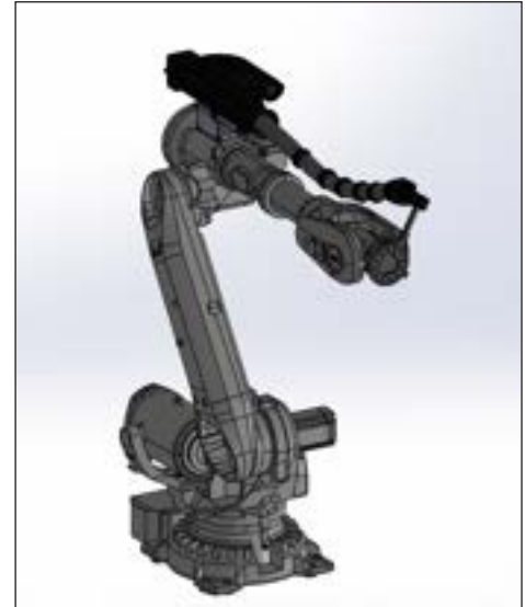
26.70.321.01 Complete robotic dresspack, Axis 3-6, TecBox retraction system, 600m stroke, high-flex conduit with ID 64mm
