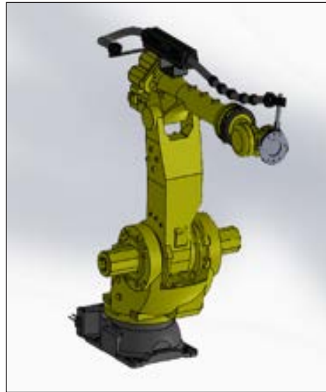
38.48.421.01 Complete robotic dresspack, Axis 3-6, TecLiner retraction system, 400m stroke, high-flex conduit with ID 36.7mm
