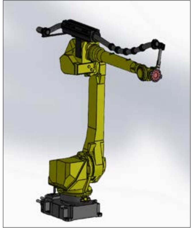
13.48.420.01 Complete robotic dresspack, Axis 3-6, TecLiner retraction system, high-flex conduit with ID 36.7mm
