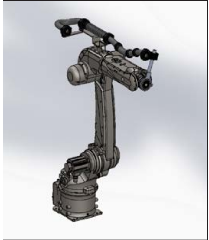
32.48.521.01 Complete robotic dresspack, Axis 3-6, external spring retraction system, high-flex conduit with ID 36.7mm
