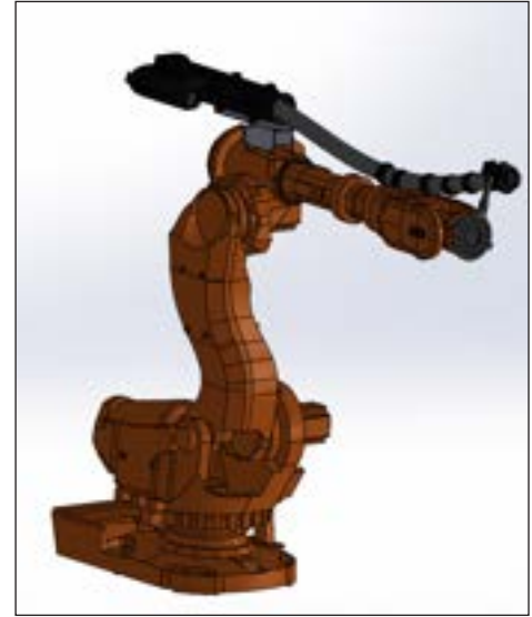
25.70.321.01 Complete robotic dresspack, Axis 3-6, TecBox retraction system, 600m stroke, high-flex conduit with ID 64mm
