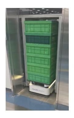
Another challenge this large manufacturer faced was an outdated automation system. Amorepacific's smart factory system installed AGV robots that had been running smoothly in its facility, when first introduced. However, as the industry entered the new age of AMR, AGV installation became outdated and less efficient than the next generation of robots–AMR.
