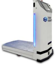
L200 has a maximum payload of 200 Kg (440.925 lbs) and a maximum speed of 1.1 m/s (2.46063 mph). It operates regardless of floor conditions, including liquids, oils, bumps, cracks, multi-levels, etc. L200 can be customized to any facility's needs.
