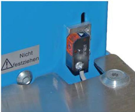
The photocell is height adjustable and used for automatic release of the banding process.
