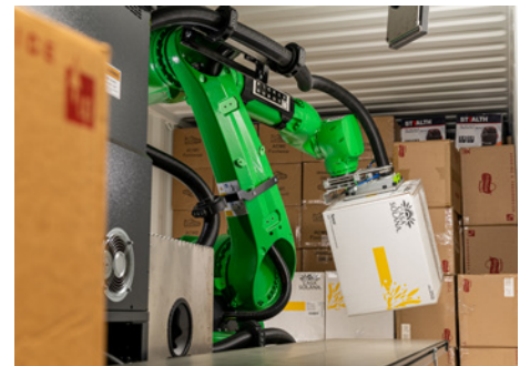
The Pickle Robot Unload System is an autonomous mobile manipulation system suitable for use with floor-loaded trailers and containers at typical dock doors.
