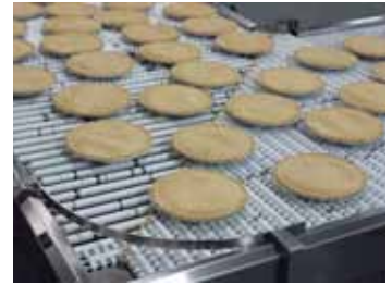
PIE FREEZER DISCHARGE TO BUFFERING PRIOR TO WRAPPER
