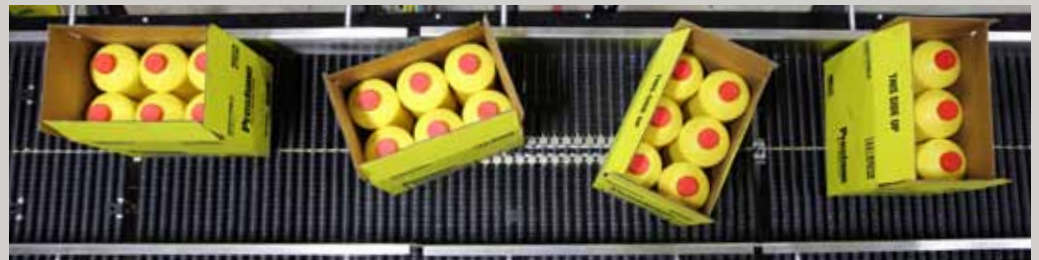
CASE ROTATOR CREATED USING A SLIP-TORQUE SPLIT-SURFACE DESIGN
