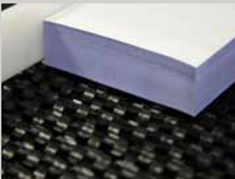
THE SLIP-TORQUE PRINCIPLE WITH STAR ROLLERS PREVENT SHINGLING OF PAPER STACKS
