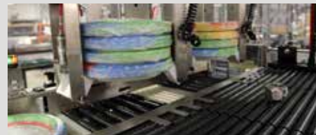
4 - PLATE BUNDLE STACKING
