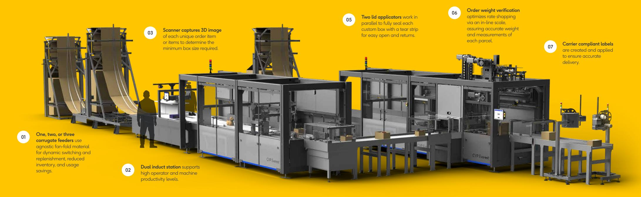
Case erector builts a fit-tosize box bottom and allows for a wide range of sizes.
