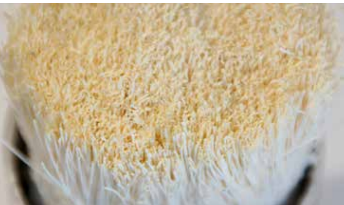
The membrane technology uses bundles of hollow fibre membranes to extract nitrogen from the ambient air.
