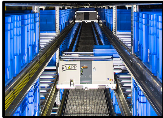
Figure 2: Fixed Rack System
