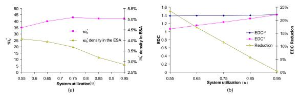
Note.  $m_e^*$  density in the ESA =  $(m_e^*/(\text{the capacity of the ESA in number of unit loads})) \times 100\%$ . Figure 6: Influence of System Utilization (*u*) on  $m_e^*$  and *EDC*
