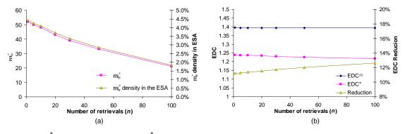
Note.  $m_e^*$  density in the ESA =  $(m_e^*/(\text{the capacity of the ESA in number of unit loads})) \times 100\%$ . Figure 3: Influence of the Number of Retrievals (i.e. Block Size *n*) on  $m_e^*$  and *EDC*
