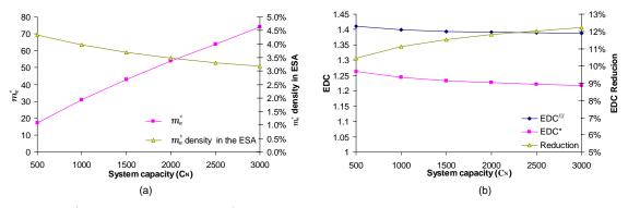
Note.  $m_e^*$  density in the ESA =  $(m_e^*/(\text{the capacity of the ESA in number of unit loads})) \times 100\%$ . Figure 4: Influence of System Capacity ( $C_N$ ) on  $m_e^*$  and EDC
