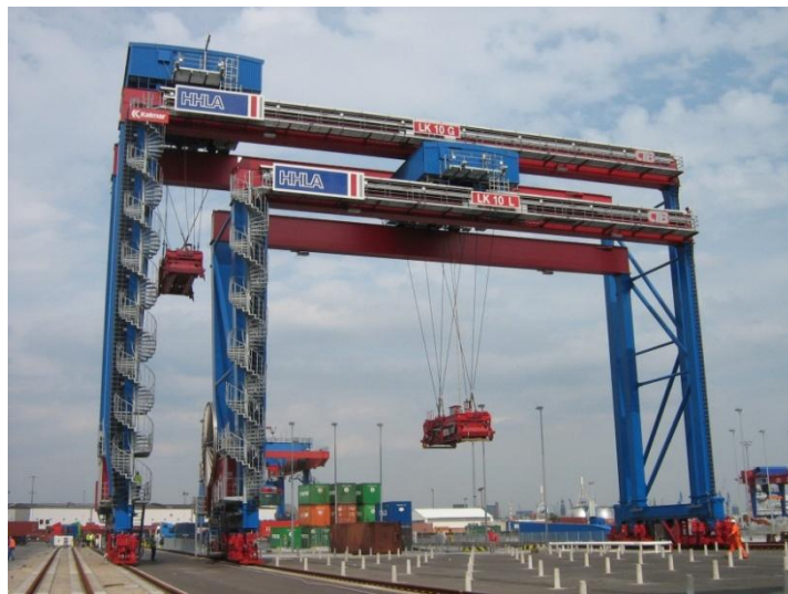
Figure 4: Passing Stacking Cranes of Kalmar Industries [8]
