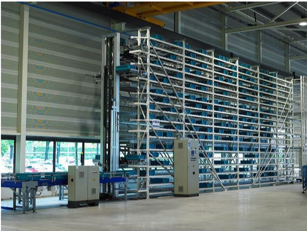
Figure 1: Dynamic storage system as developed by Vanderlande Industries (source: Vanderlande Industries)
