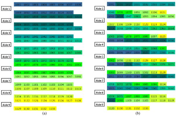
Figure 1: Assignment of SKUs to aisles using (a) demand-based method; (b) clustering method
